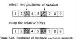
Figure 3.23. Illustration of reciprocal exchange mutation.
